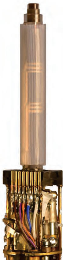
HR Liquids NMR Probe without gradient
